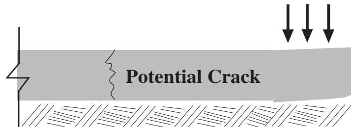
Severe slab edge curl can cause the panel edge to actually lift off the grade, creating a void beneath the panel edge. Heavy loads crossing the cantilevered panel edge may cause the panel to crack or completely break off.
