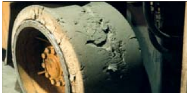
Deteriorated joints create an interruption in the continuity of the floor surface, leading to operational slow-downs and increased vehicle maintenance costs.
