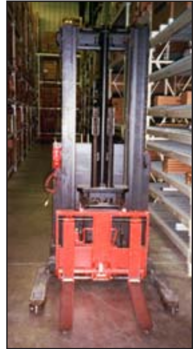
High rack lifts place higher demands on floor joints due to their smaller, harder wheels and increased point loads.
